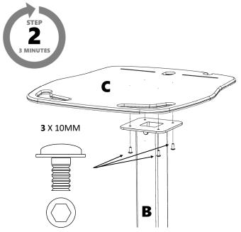
Insert and tighten the 3 x 10MM flange head fixings through the central column (B) into the work surface (C)
