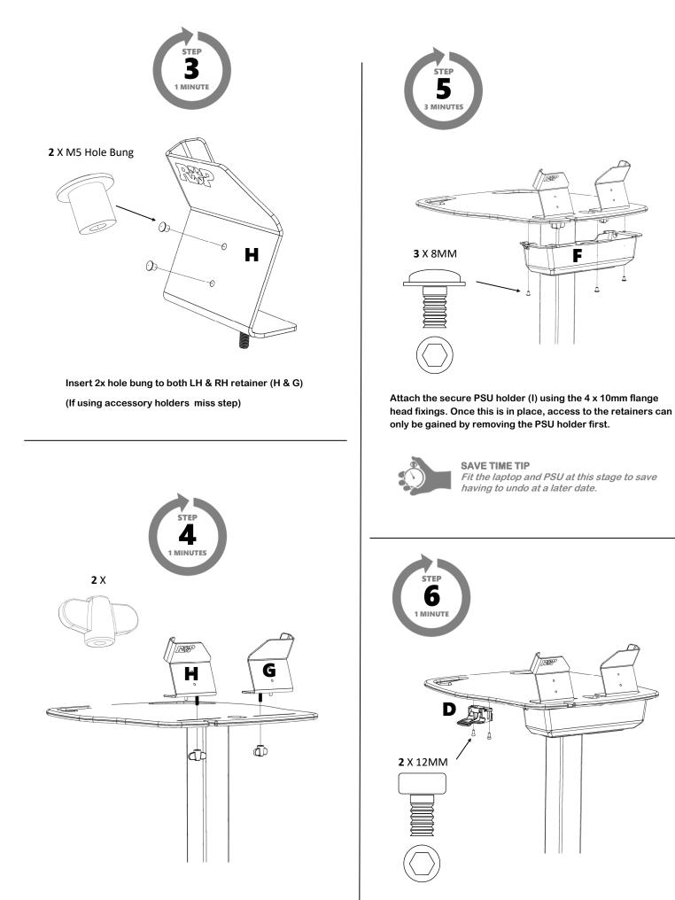
Place both retainers (H+G) into the slots\* and fix using wing nuts provided. If the laptop is to be fitted later, leave loose so the retainers can be easily moved for laptop installation.
