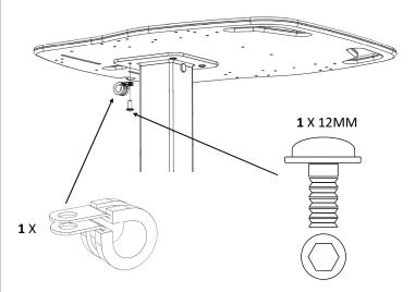
Insert and tighten the 1 x 12MM flange head fixings through Pclip then central column (B) into the work surface (C)
