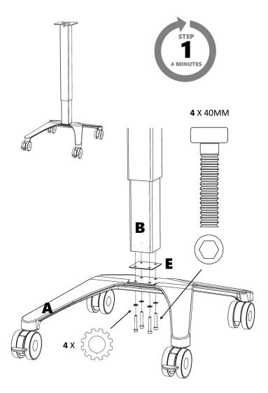
Insert and tighten the 4 x 40MM fixings with shakeproof washers through the bottom of the H-base (A), sandwiching the infill plate (E) between the central column (B)
