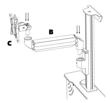
Secure connectors by tightening M4 screws with 3mm hex key provided - DO NOT OVERTIGHTEN
